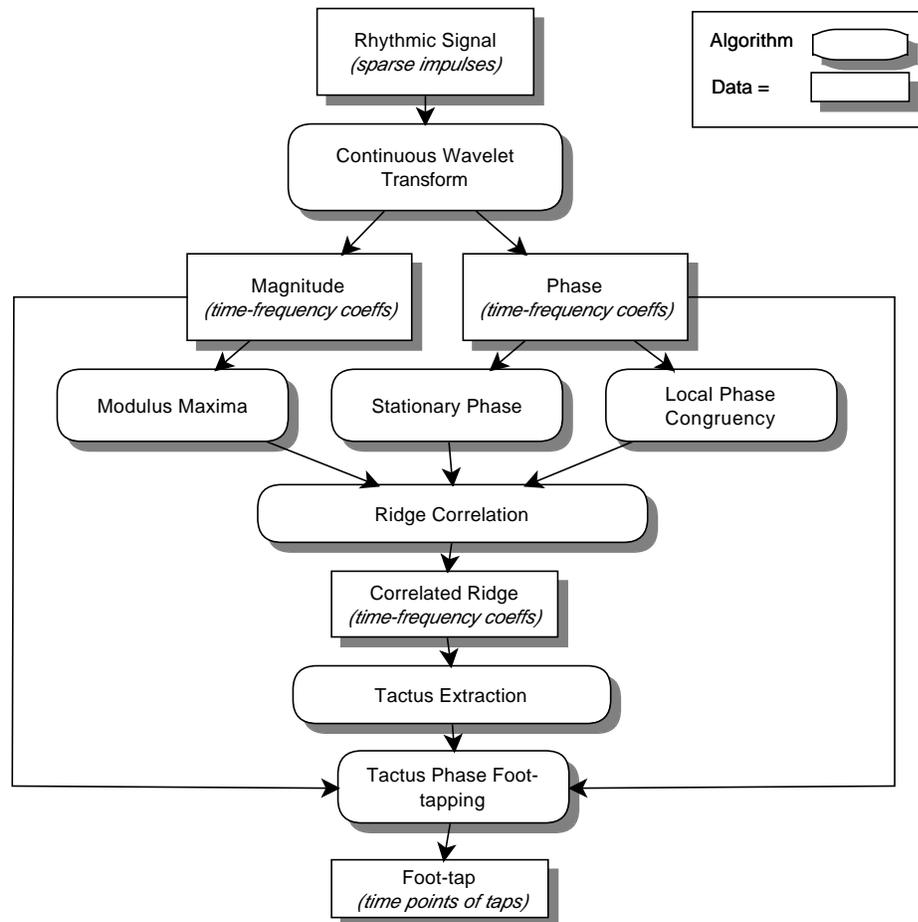
Figure 48: Schematic diagram of the multiresolution rhythm interpretation system.
