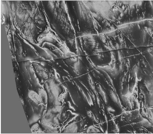
Fig. 4. Rendering of the Yilgarn aeromagnetic data using the proposed tone mapping algorithm. High-pass cutoff frequency 1/2000.
