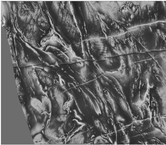
Fig. 5. Rendering of the Yilgarn aeromagnetic data using the proposed tone mapping algorithm. High-pass cutoff frequency 1/1000.
