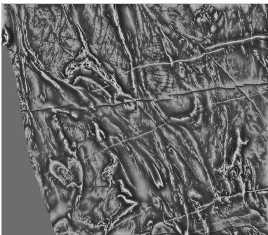
Fig. 6. Rendering of the Yilgarn aeromagnetic data using the proposed tone mapping algorithm. High-pass cutoff frequency 1/200.
