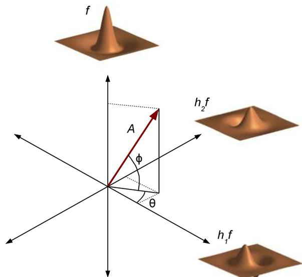
Fig. 1. Obtaining phase and amplitude from the outputs of monogenic filters. The band-pass filter is defined by  $f$ , and  $h_1f$  and  $h_2f$  are the two Riesz transform filters.  $A$  is the local amplitude,  $\phi$  the local phase, and  $\theta$  the local orientation.
