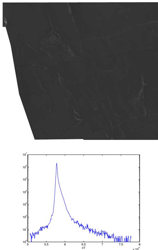
Fig. 2. Raw aeromagnetic data of the Yilgarn and logarithmic plot of its histogram values. This data is the property of Fugro Airborne Surveys Pty Ltd.
