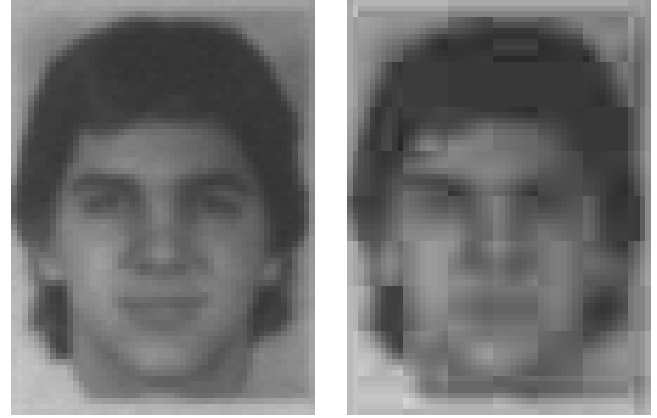
Figure 12. Further enlargement of uncompressed and 31:1 compressed face from figure 11 showing JPEG DCT blocks.
