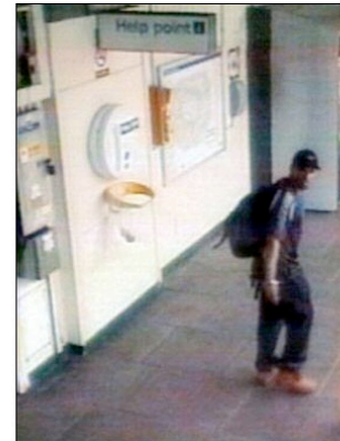
Figure 14. Images released in relation to the attempted bombings in London on July 21 2005 [2]. In the top image the letters on the jacket are about 80-90mm high, assuming the head is 160mm wide. They are not legible. In the second image the 'Help Point' letters on the overhead sign are larger still, yet only just legible. It might be argued that these surveillance cameras are legally blind!
